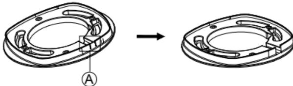
3. Loosen the screws with the tamper-resistant hex wrench (supplied) to remove the camera cover.
