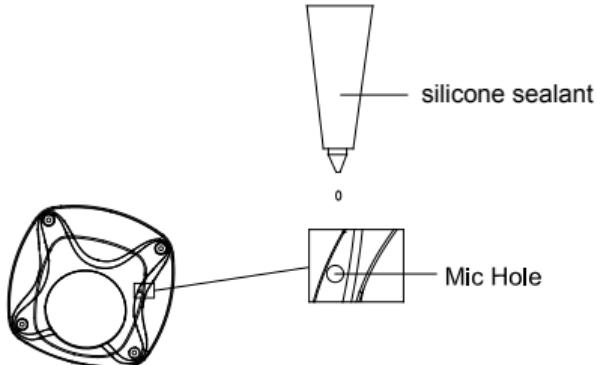
When installing the camera in a corrosive environment, such as marine ships, coastal sites, or chemical factories, please use silicone sealant (purchased separately) to seal the microphone hole. The typical cure time is about one to two hours in the temperature range between 40 and 100°F (5 and 40°C).
