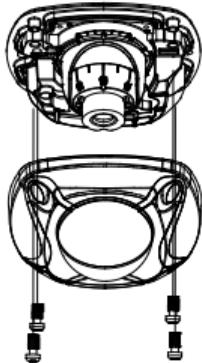
4. Mount the camera base to the converter pan or mounting surface, depending on the installation.
