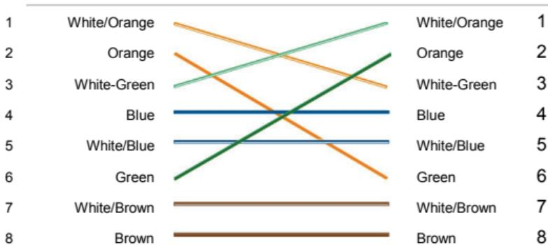
Please make sure your connected cables have the same pin assignment and color as above before deploying the cables in your network.
